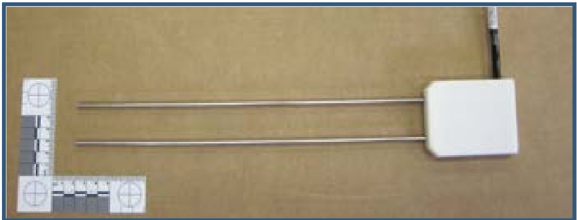
Figure 20: Time domain reflectometer (TDR)
