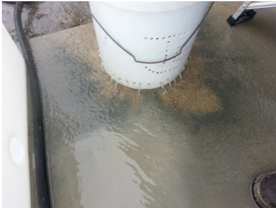
Figure 16: Washing the aggregate using a pressure washer
