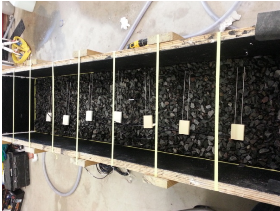
Figure 21: Arrangement of TDRs in the storage gallery
