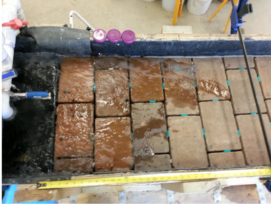
Figure 45: Experiment #19, 5% slope, 6 mm gap size, no aggregate between the pavers
