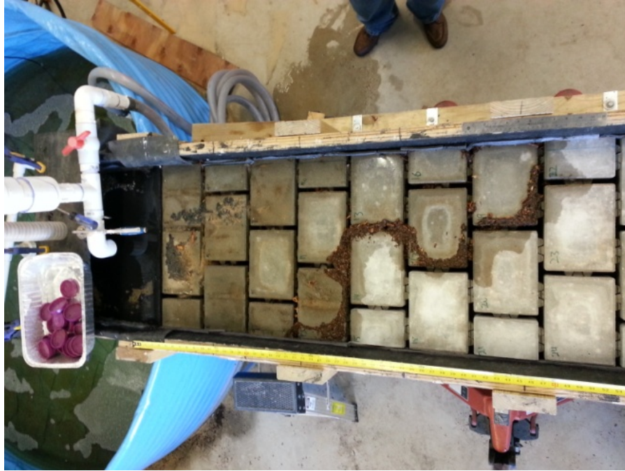
Figure 34: Experiment #7, 1% slope, 12 mm gap size, no aggregate between the pavers
