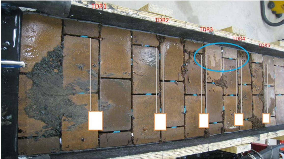
Figure 62: Flume's overview for progression of clogging in experiment #1
