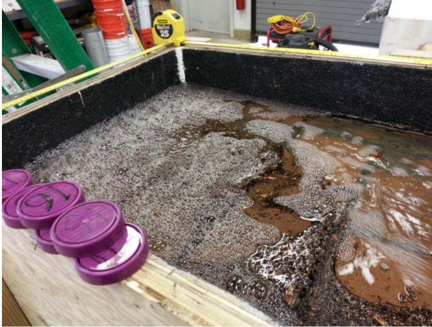
Figure 41: Clogged but not sealed, experiment #18, 5% slope, 9 mm gap size, #8 aggregate between the pavers
