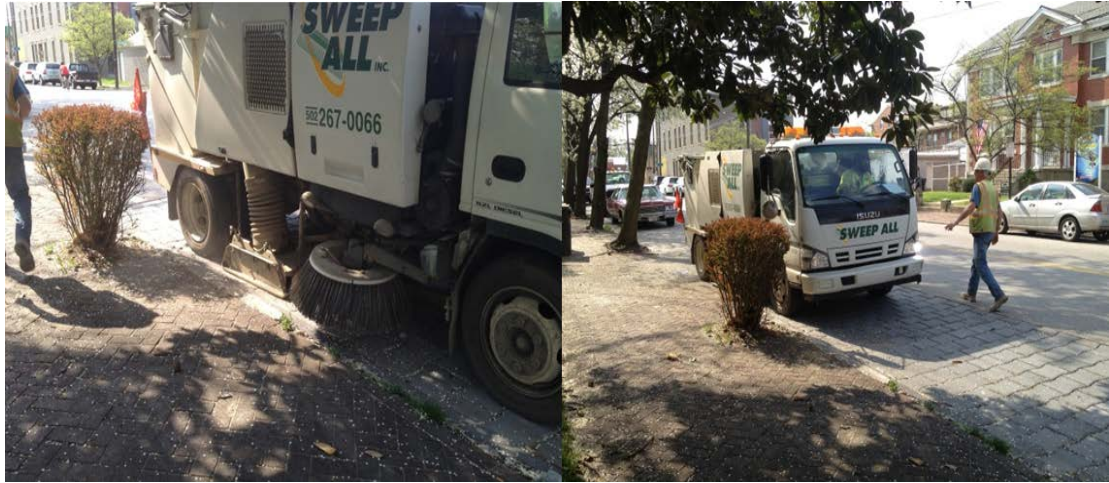
Figure 4: Regenerative sweeper truck with NQR 435 vacuum chamber (53 hp)
